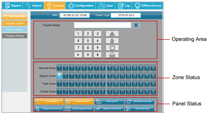
Figure 5-41 Keypad Control (23 Series Panel)
